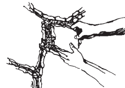
Figure 10 Position large pieces first, then trim and fit in smaller pieces.
