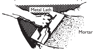
Figure 5 Apply mortar using a plasterer's trowel.
