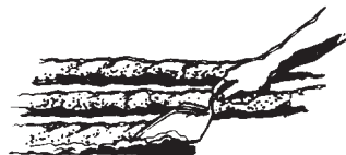
Figure 16 Place mortar for Hearthstone installation.
