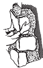
Figure 8 Apply corners—alternating long and short legs in the opposite directions.
